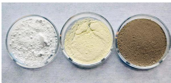
*The picture illustrates the difference in colour of the doped powders in comparison to a pure white sample of  $TiO_2$ . The white sample to the left sample is P25 Evonic, The light yellow sample in the middle is the (N, S) doped DNT1th powder, and the brownish sample to the right is the (N, Ag) doped DNT1\_Ag.*
