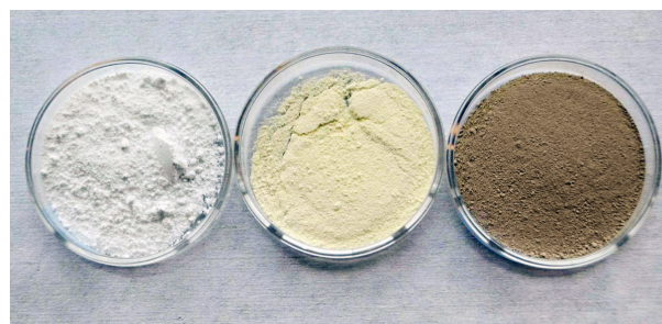
The picture illustrates the difference in colour of the doped powders in comparison to a pure white sample of \text{TiO}_2 . The white sample to the left sample is P25 Evonic, The light yellow sample in the middle is the (N, S) doped DNT1th powder, and the brownish sample to the right is the (N, Ag) doped DNT1_Ag.
